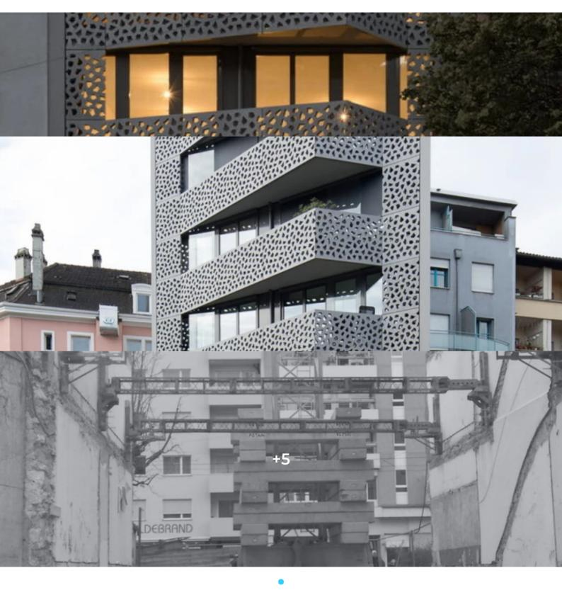
The signature symbol of the building are the prefabricated perforated glass-reinforced concrete elements of both facades, combined with the large glass surfaces lying underneath, as well as the angled geometry of the balconies. These building blocks give the project a modern look.
